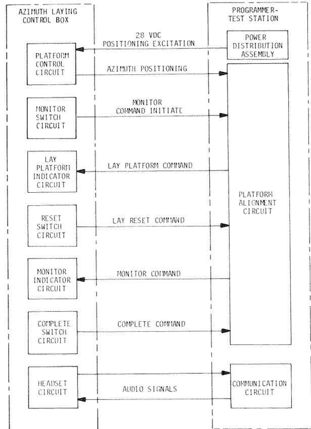
**Figure 6-6. Azimuth Laying Control Box Signal Flow Diagram**
