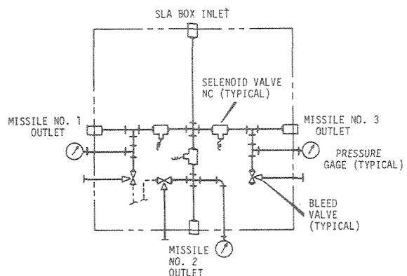
Figure 11-16. High Pressure Air Switching Schematic
