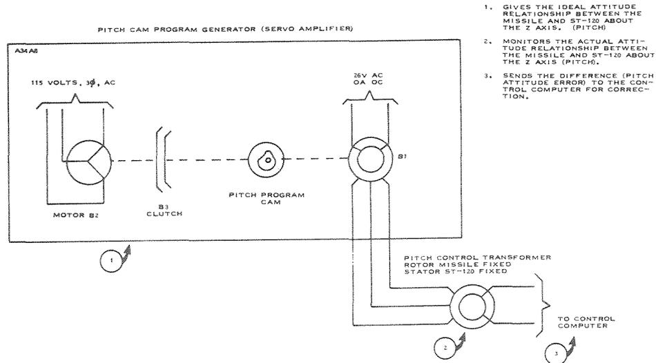
Figure 2-28. Pitch Cam Program Generator
