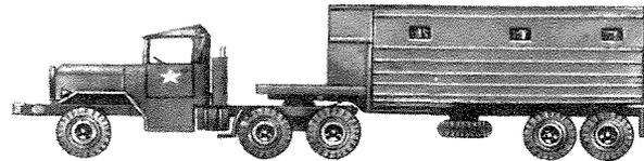
***Figure 1-12. Typical Maintenance Shop and Supply Van***
