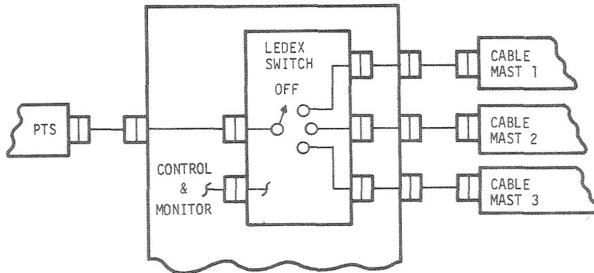
Figure 11-15. Typical One-Line SLA Connection Diagram
