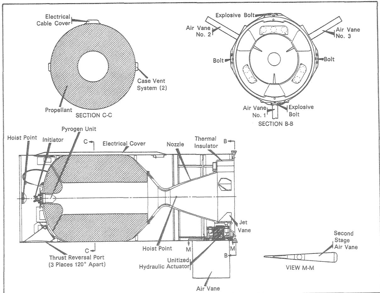
Figure 2-5. Second Stage Motor Section, Inboard Profile
