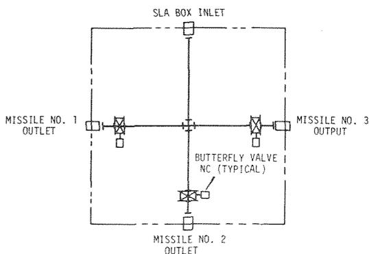
**Figure 11-17. SLA Conditioned Air Switching Schematic**
