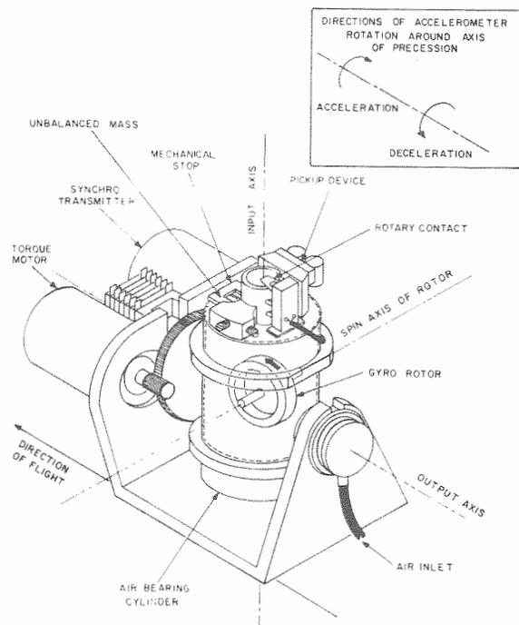
**Figure 2-23. Integrating Accelerometer**
