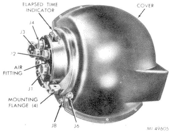
**Figure 2-15. ST-120 Inertial System**
