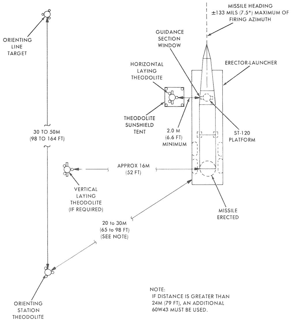
Figure 6-8. Typical Emplacement of Azimuth Laying Set
