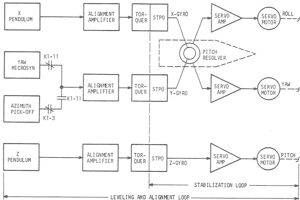
Figure 2-25. ST-120 Stabilization and Alignment Loop, Missile Horizontal
