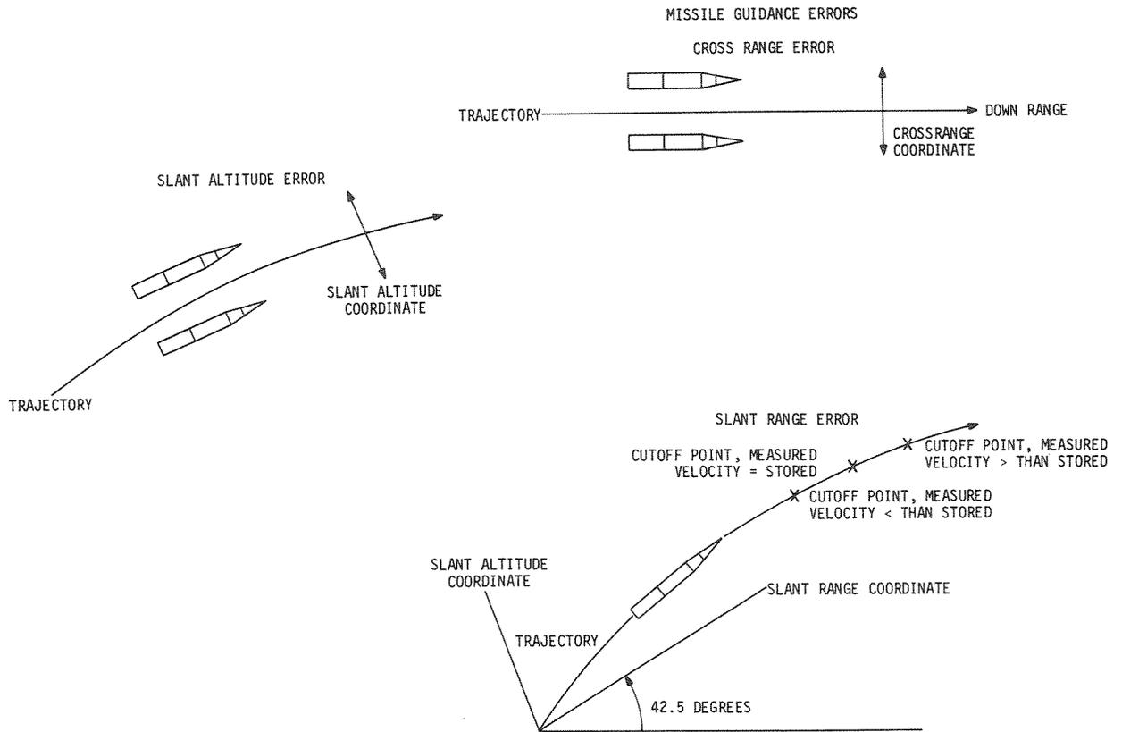
**Figure 2-8. Missile Guidance Coordinates and Errors**
