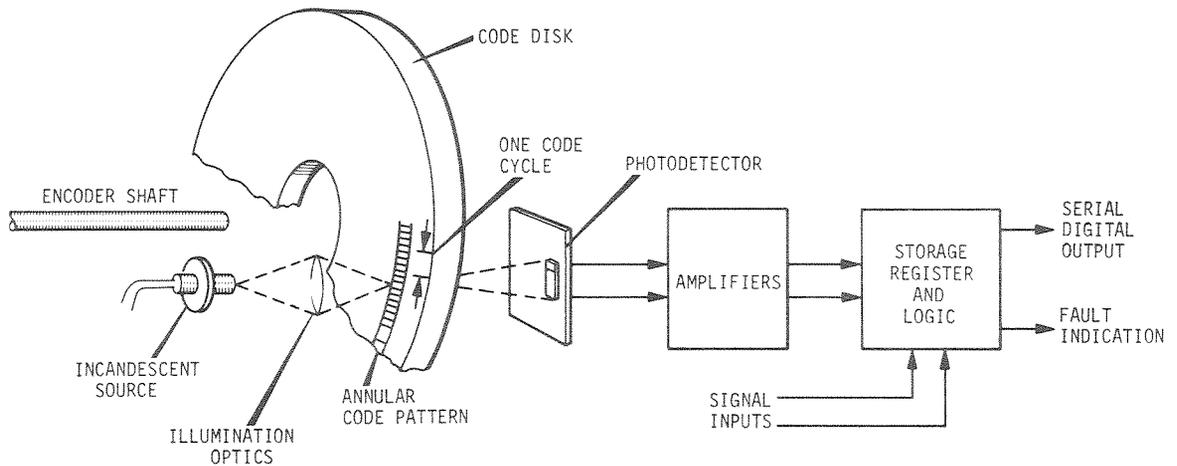
Figure 11-6. Digital Encoder Functional Schematic
