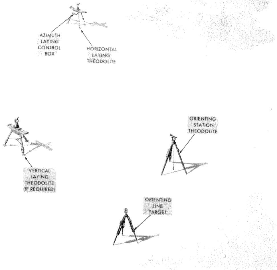
*Figure 6-1. Principal Components of the Azimuth Laying Set*
