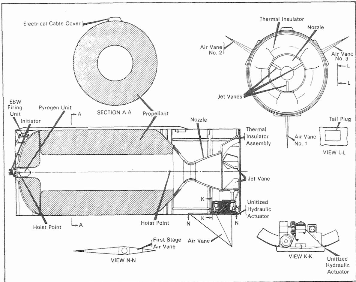
**Figure 2-4. First Stage Motor Section, Inboard Profile**
