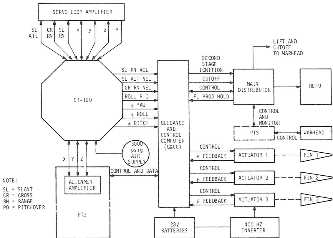
Figure 2-7. Guidance and Control System Functional Schematic
