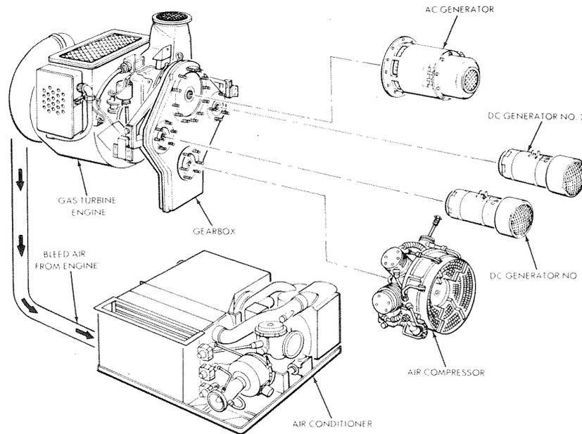
**Figure 5-4. Engine Powered Assemblies**
