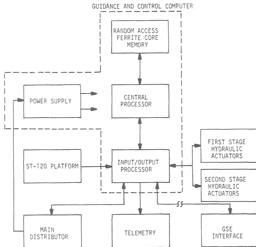
Figure 2-31. Guidance and Control Computer System Organization
