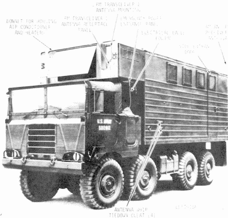
*Figure 7-3. BCC Three Quarter Front Exterior View*
