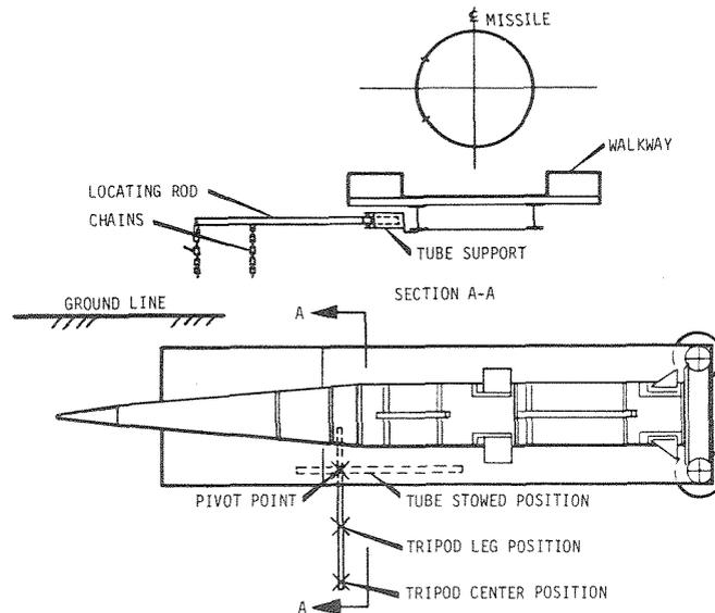
**Figure 11-12. Tripod Emplacement Device**
