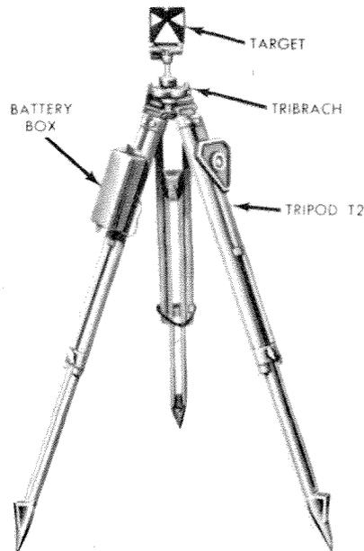
Figure 6-4. Orienting Line Target
