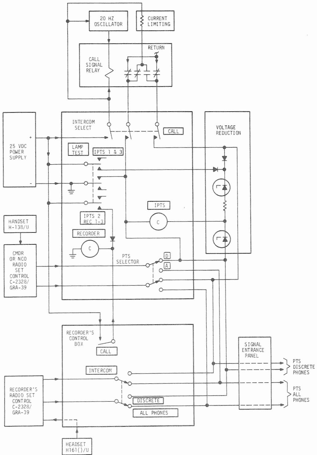
Figure 7-2. BCC/PTS Typical Intercommunications Schematic
