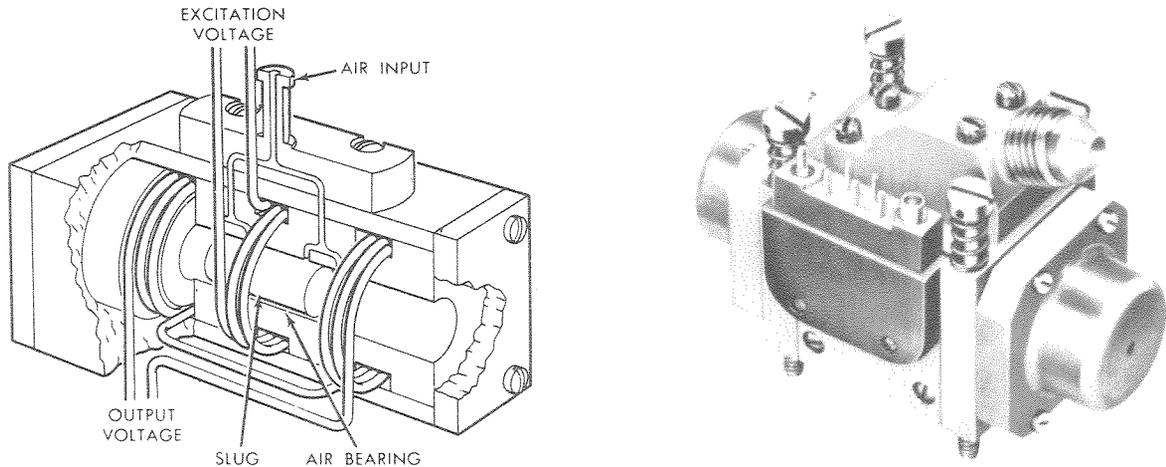
Figure 2-24. Air Bearing Pendulum
