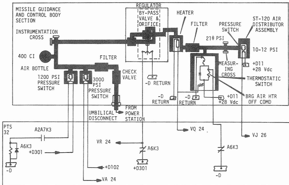
Figure 2-30. Air System Functional Diagram
