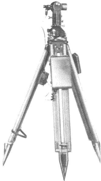
**Figure 6-3. Orienting Station Theodolite**
