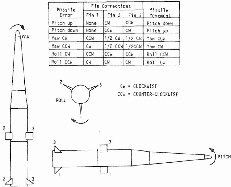
Figure 2-10. Missile Response to Attitude Errors
