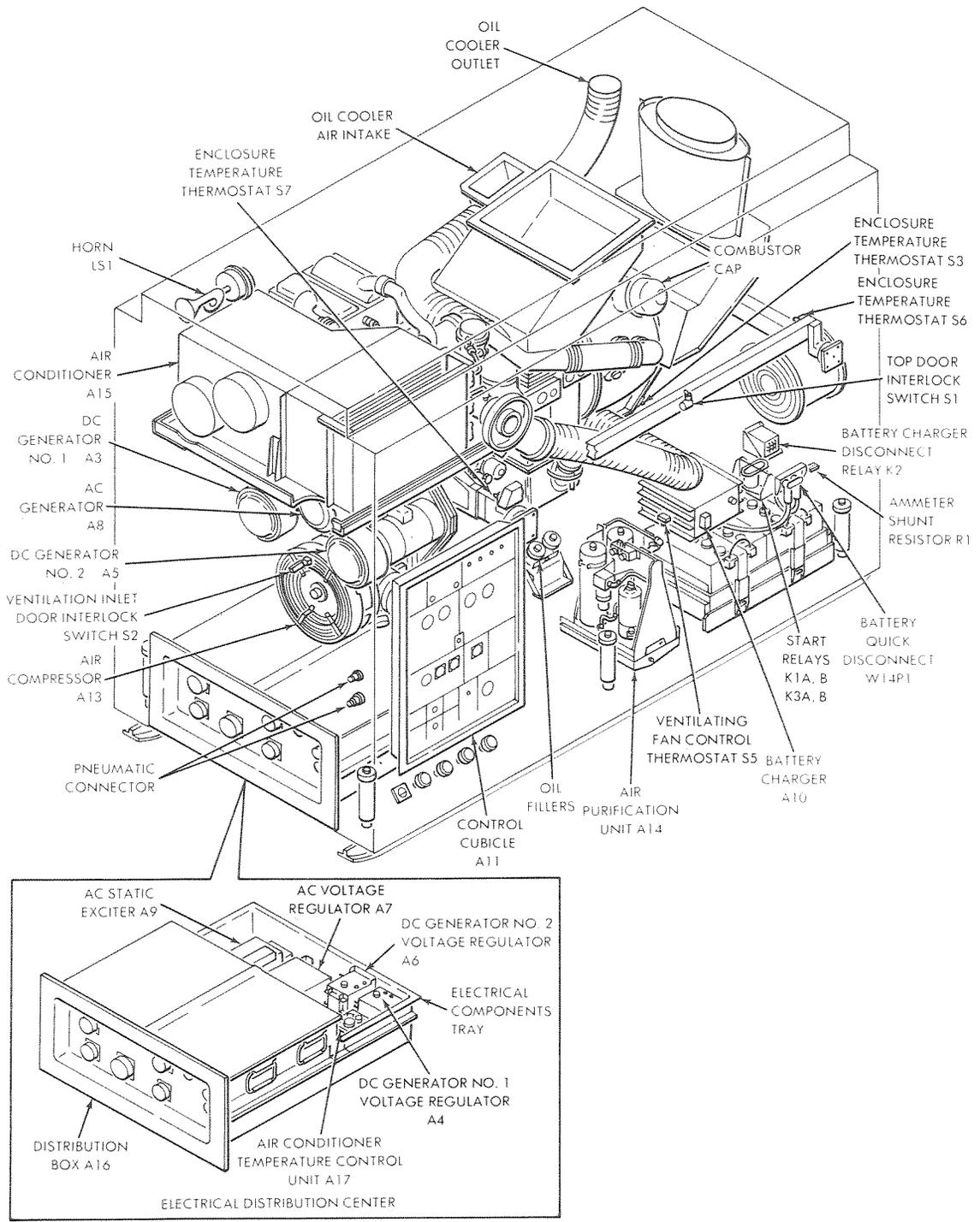
Figure 5-2. PS Three Quarter Front Internal View
