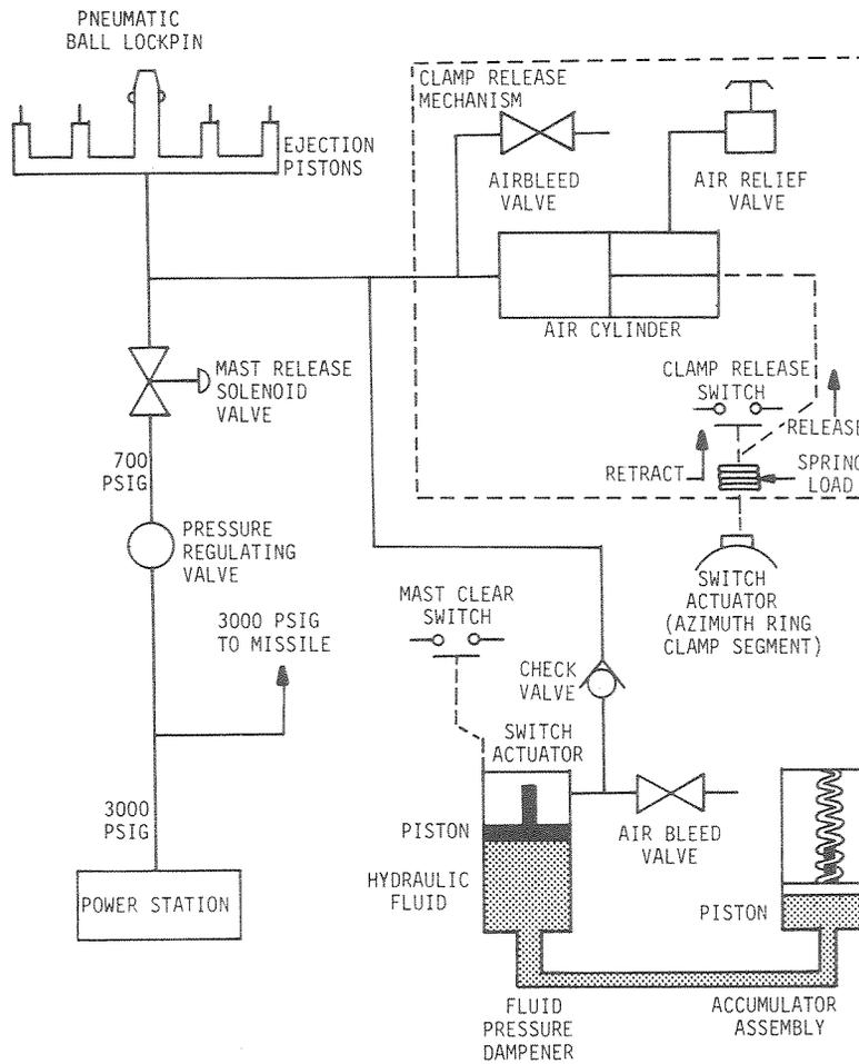
Figure 3-11. Cable Mast and Clamp Release Mechanism Pneumatic Diagram
