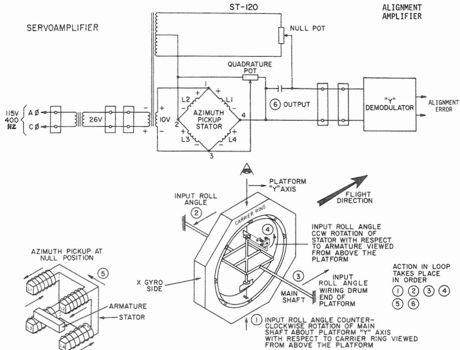
Figure 2-26. Azimuth Pickoff Operation
