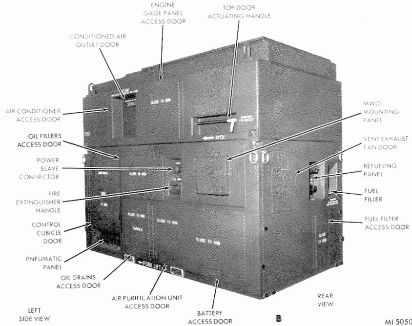
Figure 5-1. Power Station Enclosure, Three Quarter Front and Rear Views
