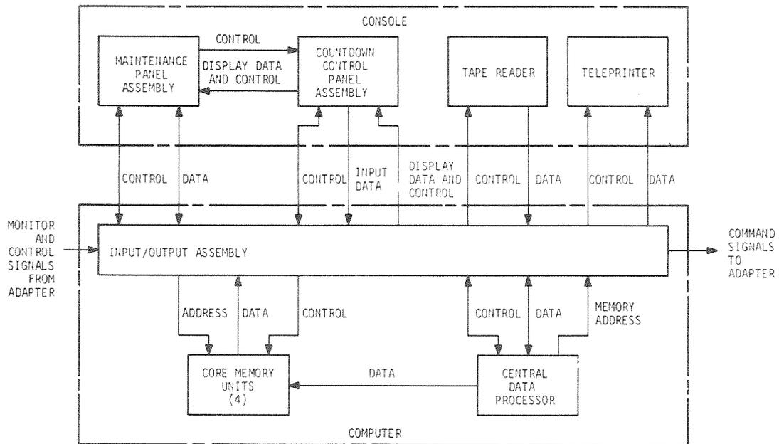
Figure 4-5. Computer Block Diagram
