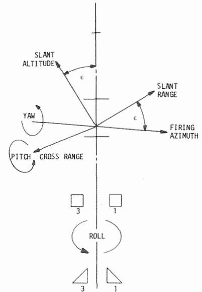
Figure 2-11. Missile Coordinate System
