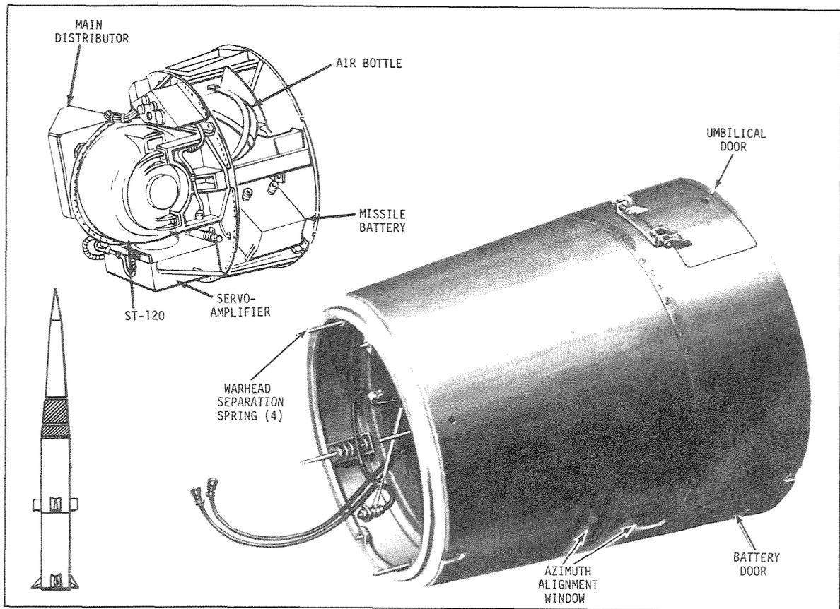
*Figure 2-6. Guidance and Control Section*
