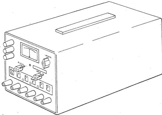
*Figure 10-10. AC/DC Differential Voltmeter*
