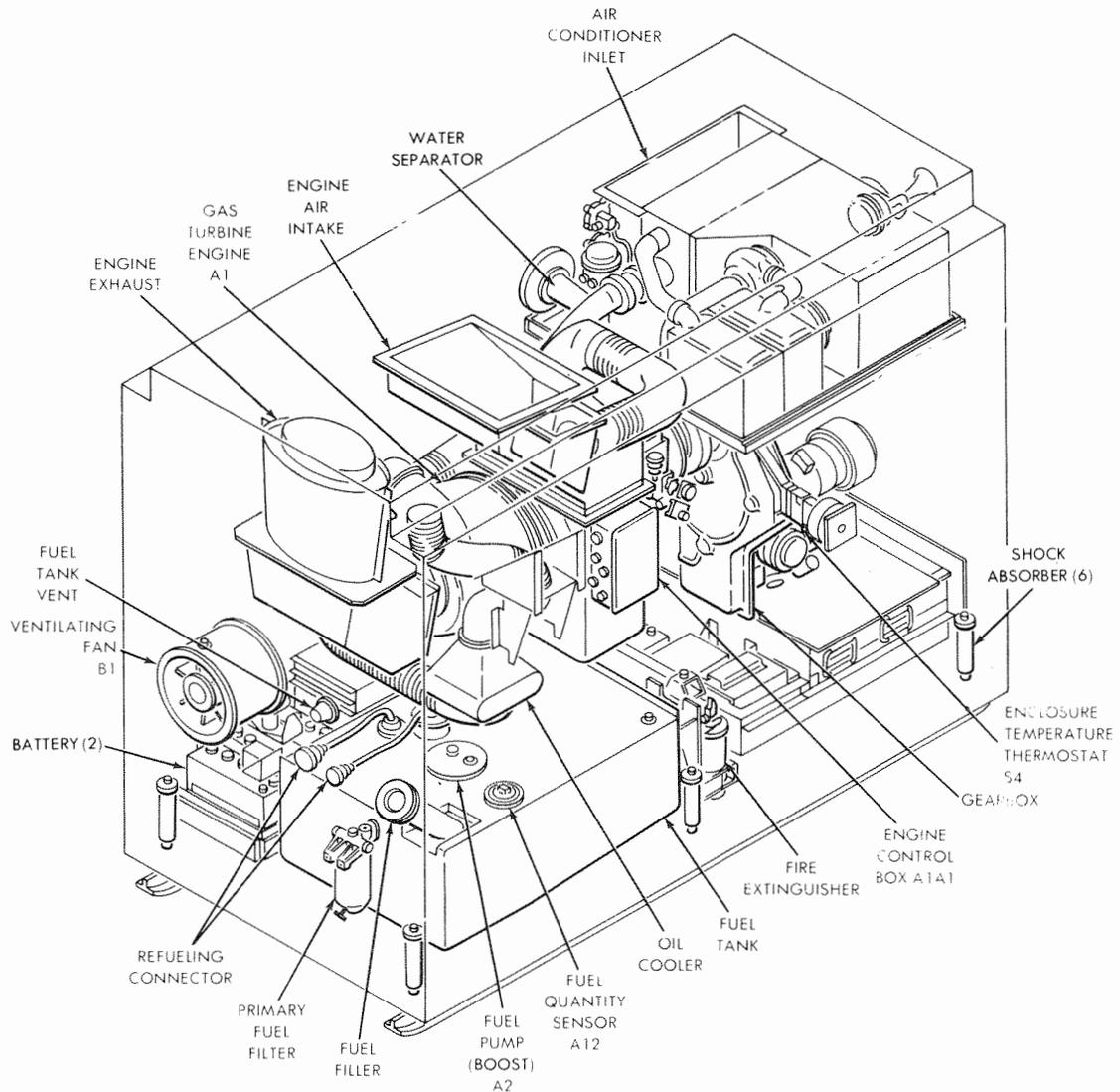
*Figure 5-3. PS Three Quarter Rear Internal View*
