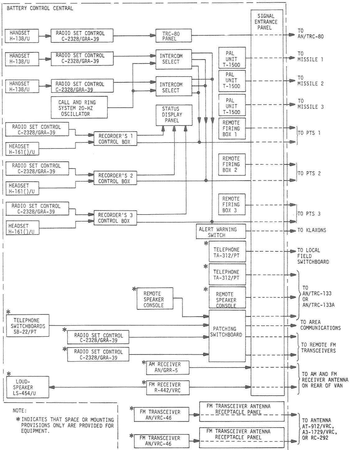
Figure 7-1. Battery Control Central Equipment Block Diagram
