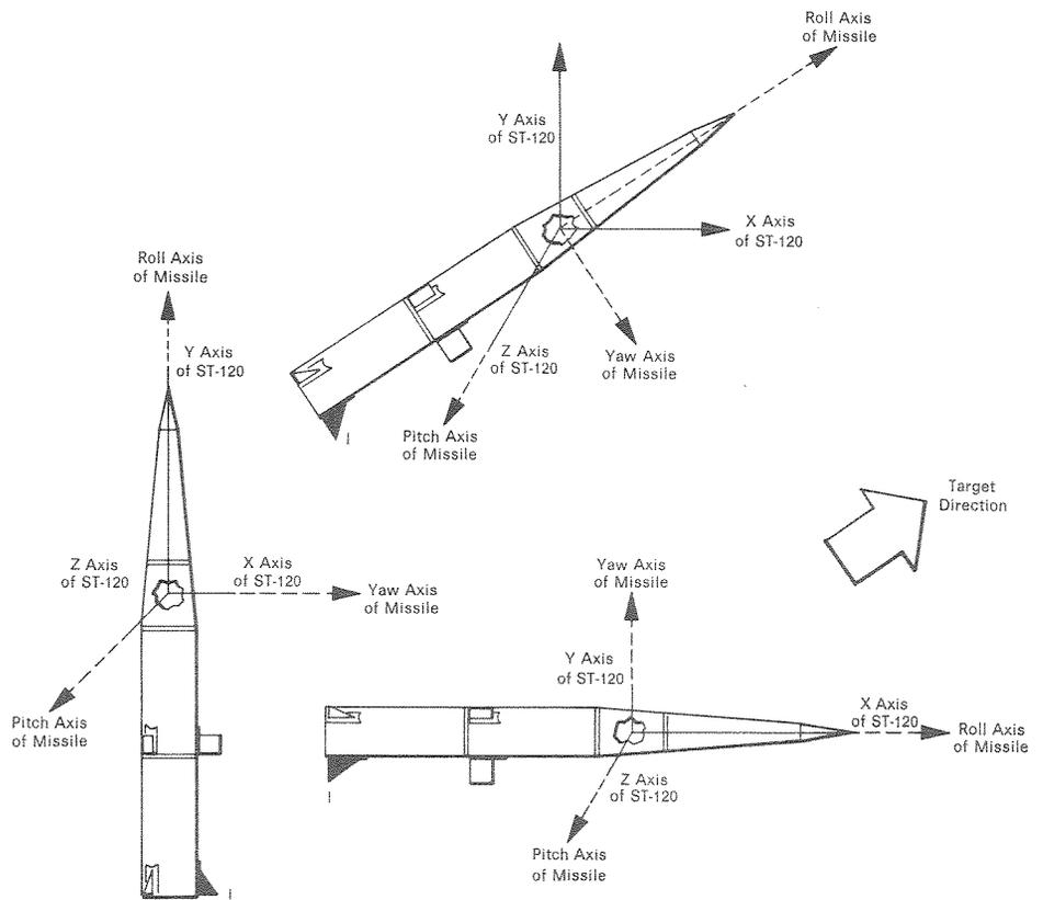
**Figure 2-16. ST-120 Missile Axes Orientation**
