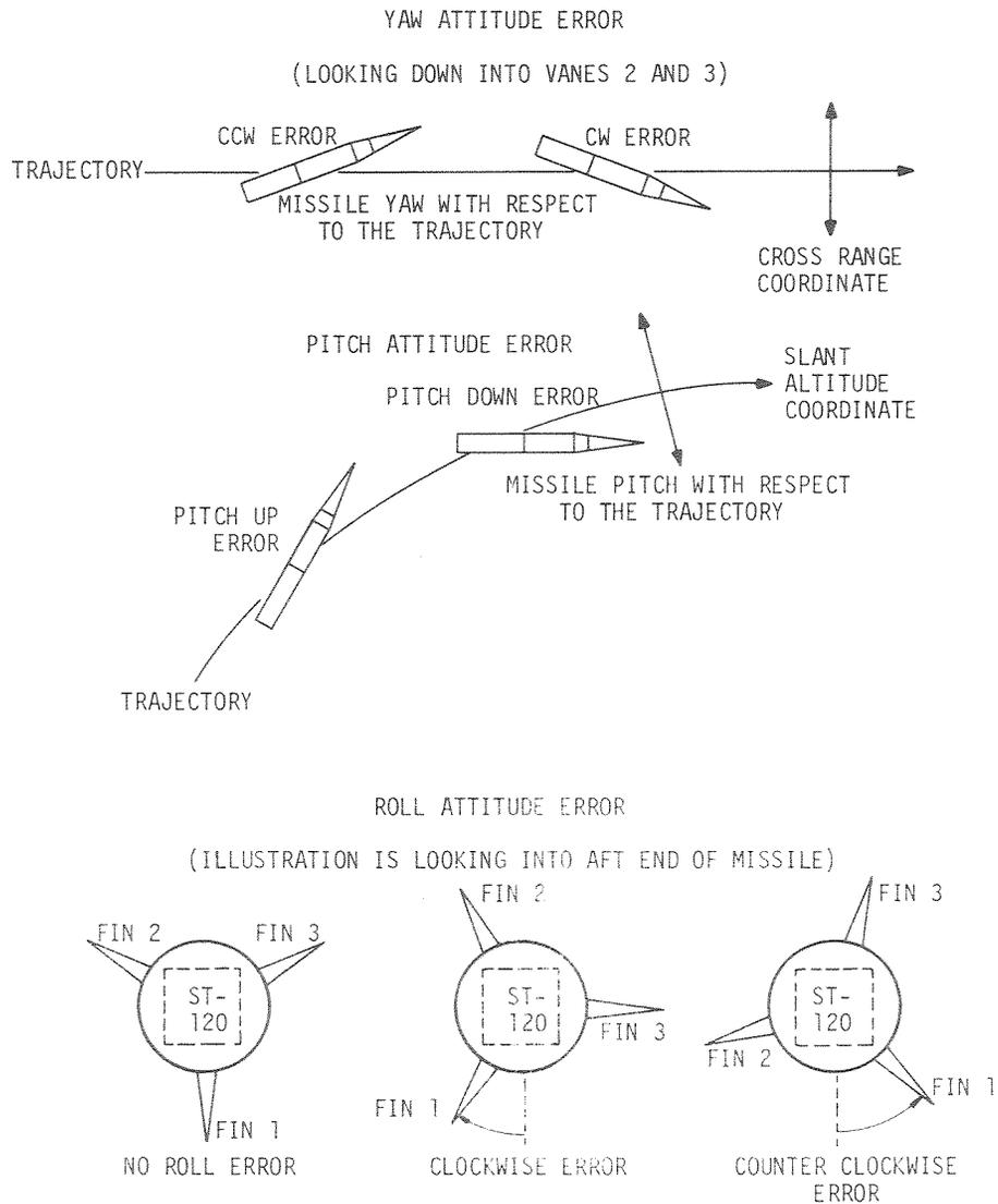
*Figure 2-9. Missile Attitude Errors*
