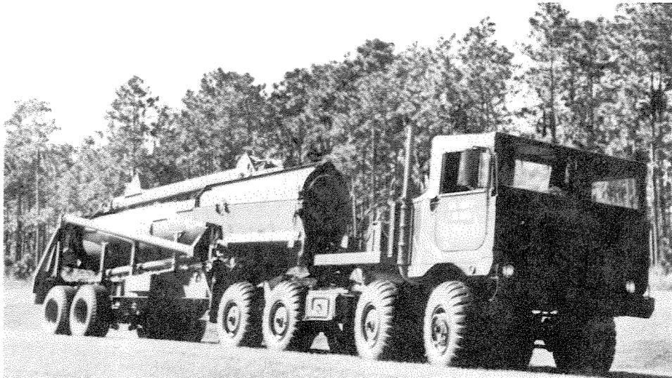
***Figure 1-4. Tractor with Erector-Launcher***
