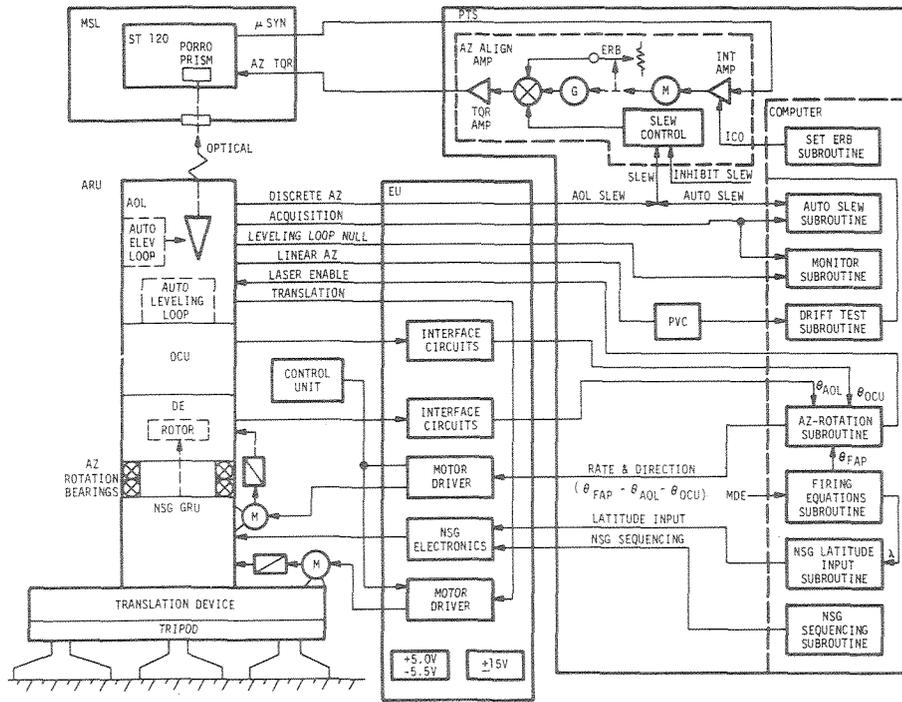
Figure 11-4. ARS Block Diagram
