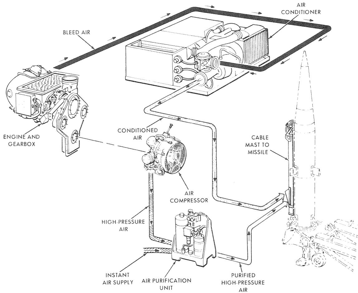
Figure 5-5. Air System Flow Diagram
