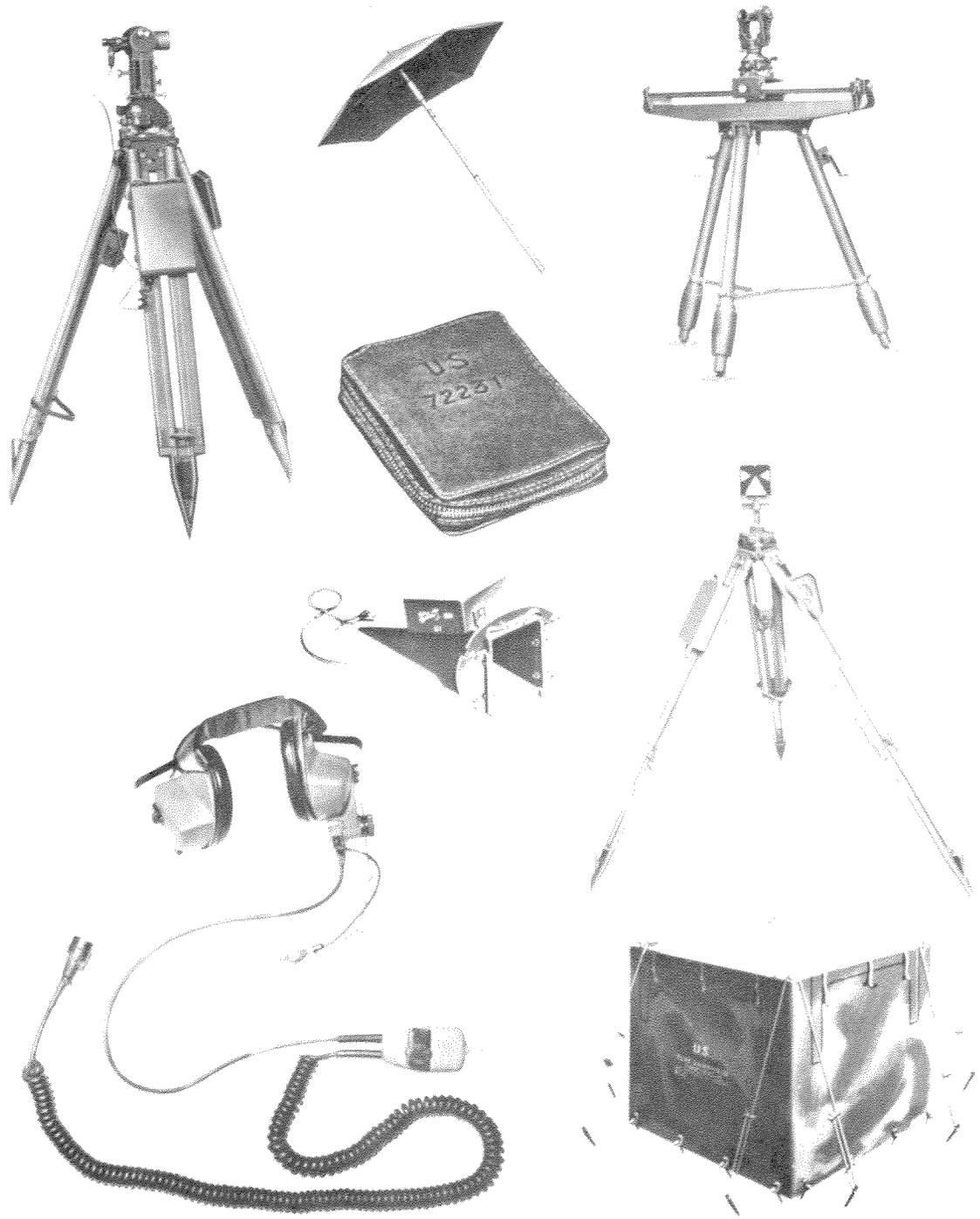
*Figure 1-6. Azimuth Laying Set*
