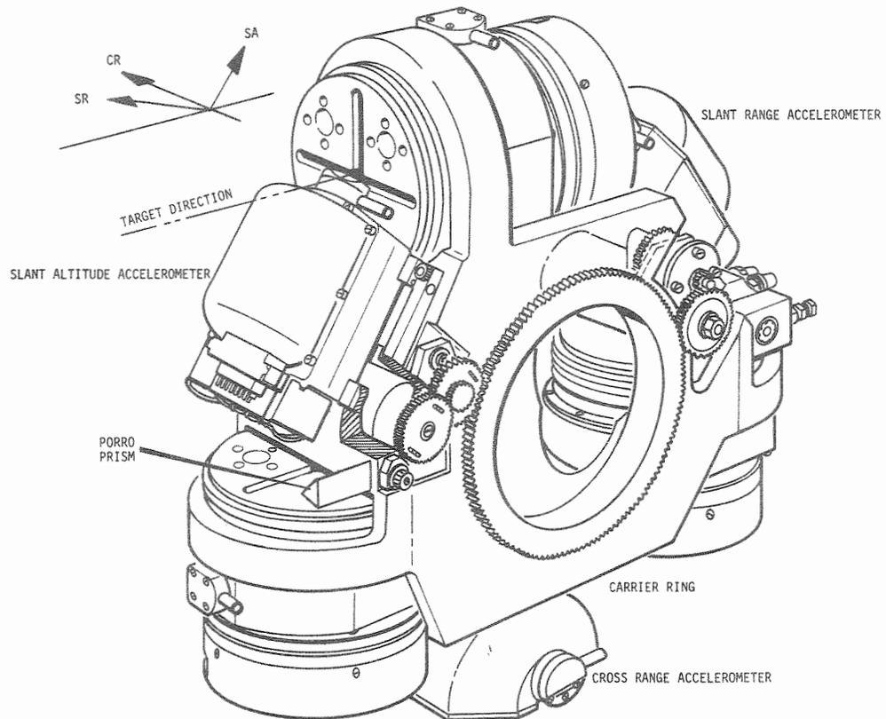
Figure 2-19. ST-120 Accelerometer Orientation and Subassembly Location
