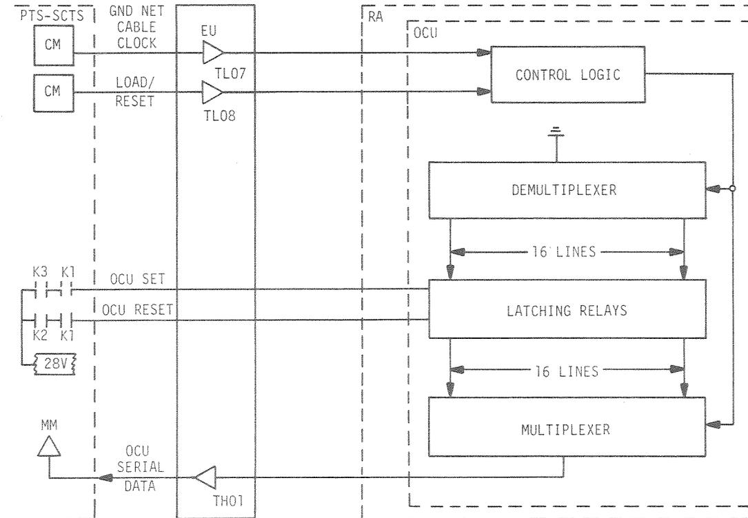
Figure 11-7. Offset Correction Unit Block Diagram
